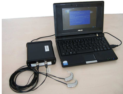
Figure 3: PHS prototype based on the Asus Eee PC, with a dimension of 22 \times 15 cm and a weight of 1.2 kg, including the sound card and audio headsets.
